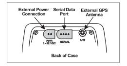
To connect the unit to an external power source, plug the included power cable into the connector labeled "Power." Connect the cable to a 6VDC to 32VDC power source. Note that the unit will use external power if the voltage from the external source is higher than the internal battery voltage.
